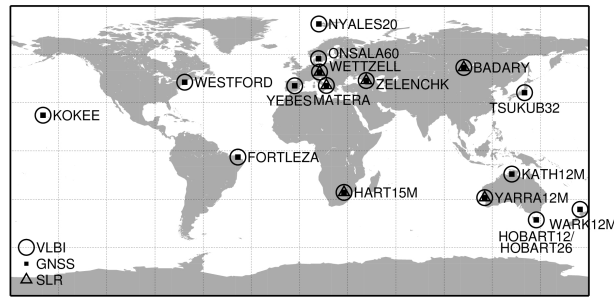
Fig. 2.3: CONT14 station map: VLBI stations ( circle ) and co-located techniques for each site ( square = GNSS, triangle = SLR); a detailed station list is given in Tab. C.1
