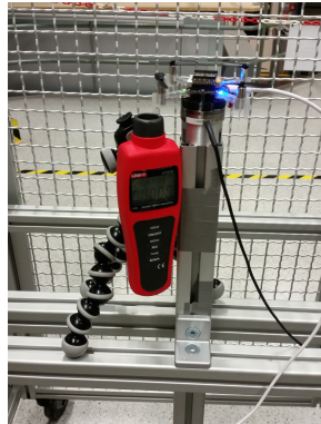
Figure 3.5: Mounting position of the tachometer. It is fixed to the aluminium profiles using a tripod.
