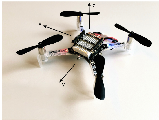
Figure 2.4: Crazyflie together with the body frame that was defined. The x axis corresponds to the pitch, y to the roll and z to the yaw axis of the quadcopter. This coordinate system is referred to throughout the whole report.
