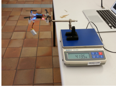
Figure 3.8: Experimental setup that was used to verify that the load cell provides correct values for the thrust produced by the Crazyflie.
