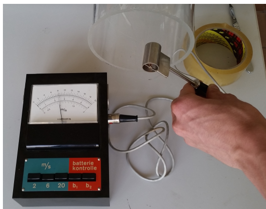
Figure 4.5: Anemometer that was used to determine wind velocities.
