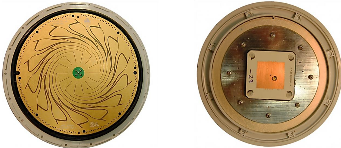
Figure 3.20 Pinwheel™ antenna Leica ATX1230 GG (left) and patch antenna Leica 500 (right). (Photos: D. Grimm)
