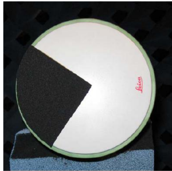
Figure 7.13 Leica ATX 1202 GG antenna with stuck on attenuating material (Zeimet, 2009)
