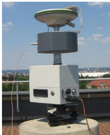
Figure 7.11 NORDIS mounted on DRB2 at TU Dresden. (Picture: D. Grimm)
