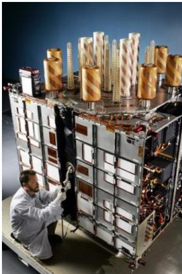
Figure 3.15 Helix antennas mounted on a GPS-Block-2 satellite (Lockheed Martin, 2005).
