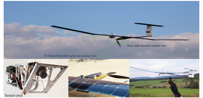
Fig. 10: The AtlantikSolar UAV with the sensor pod attached to its wings and further photos of the sensor pod, the solar cells and an instant of the hand-launching.
