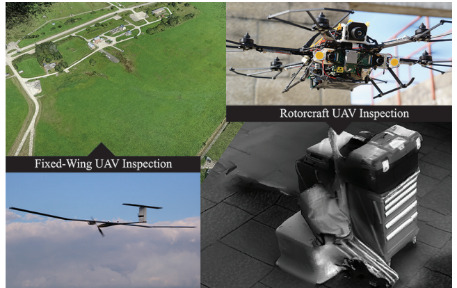
Fig. 1: Indicative inspection 3D reconstruction results using the proposed structural inspection planner and a rotorcraft as well as a fixed-wing UAV equipped with camera sensors.
