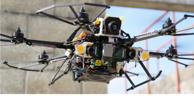
Fig. 8: The Firefly UAV equipped with the VI-Sensor.
