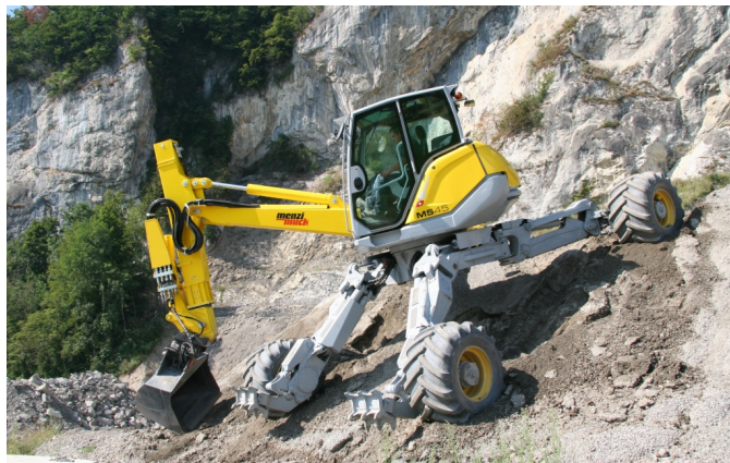
Fig. 1: Walking excavators are deployed for work in challenging environments.
