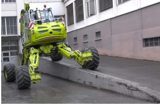
(a) Experimental setup for driving up and down a ramp.
