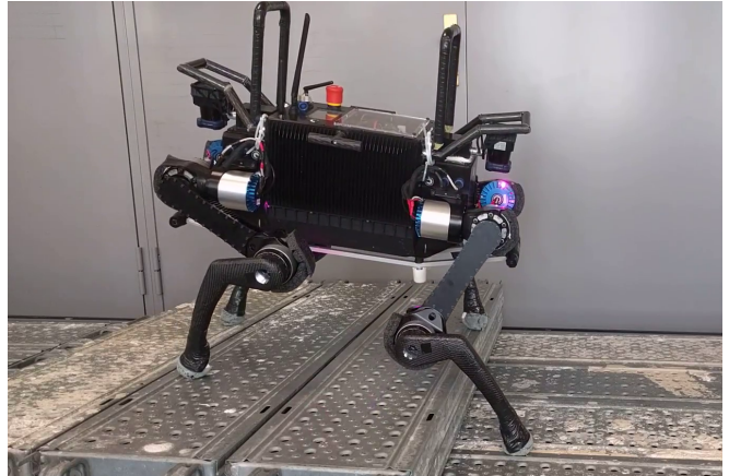
Fig. 1. ANYmal is a fully torque-controllable quadrupedal robot, actuated by custom developed series elastic actuators which provide very precise torque control.
