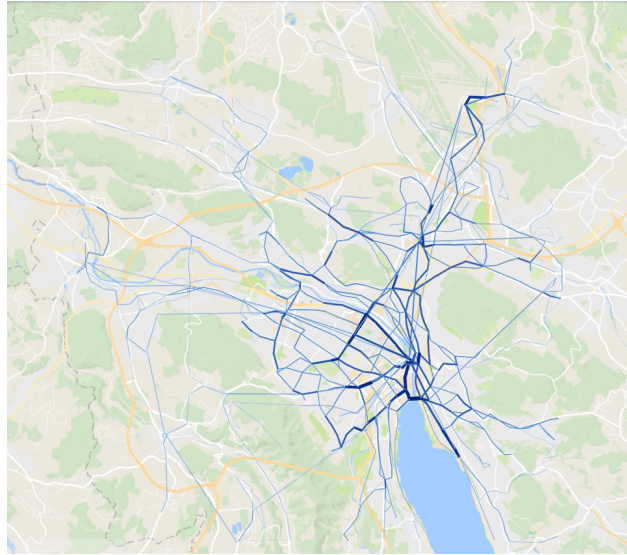
Figure 6: Public transport traffic in Zürich: darker and larger lines represent more transport vehicles travelling on a working day (26-03-2018).
