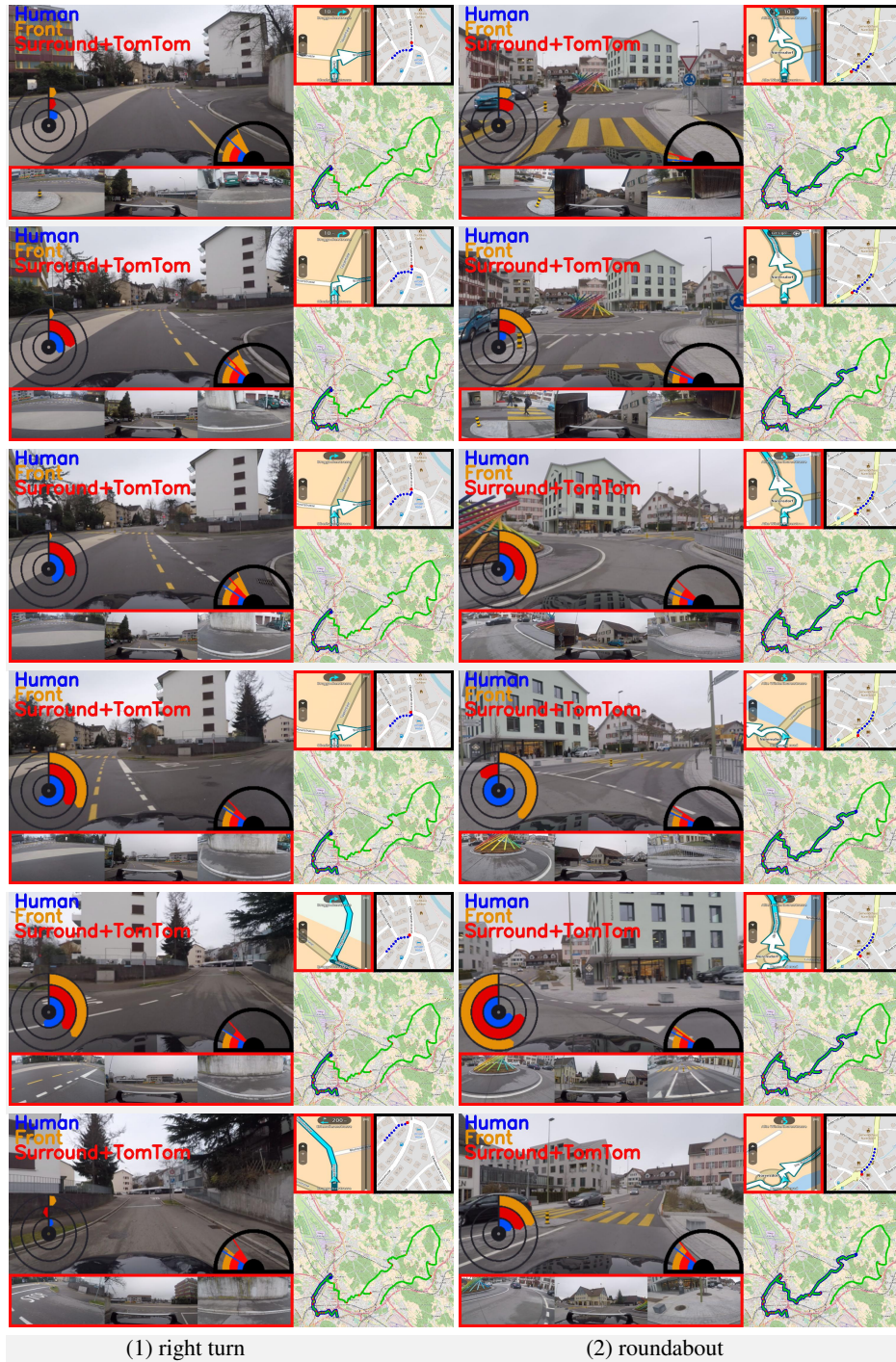
Fig. S3: Qualitative evaluation of Surround-View + TomTom and Front-Camera-Only models. Example for two driving maneuvers: (1) right turn (2) roundabout, with a sequence of temporal frames. Better seen on screen.
