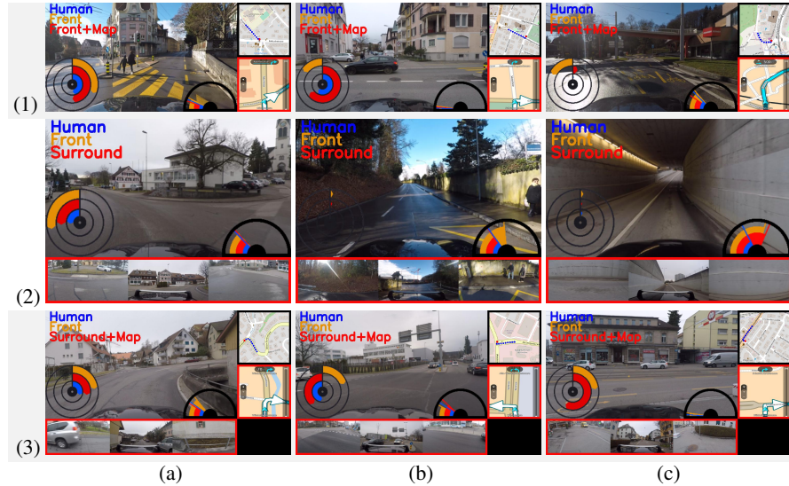
Fig. 3: Qualitative results for future driving action prediction, to compare three cases to the front camera-only-model: (1) learning with TomTom route planner, (2) learning with surround-view cameras (3) learning with TomTom route planner and surround-view cameras. TomTom route planner and surround-view images shown in red box, while OSM route planner in black box. Better seen on screen.
