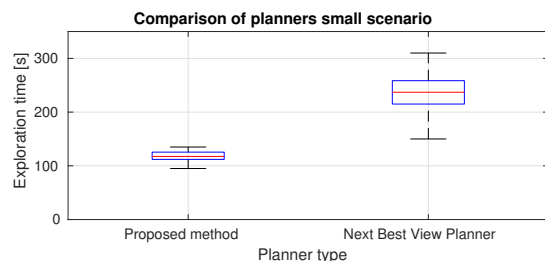
Fig. 7. The boxplot for 20 exploration runs in the small scenario with our planner without history and [6] at the same maximum velocity V_{max} = 1.2\text{ms}^{-1} . Our improvements clearly reduces the exploration time and variance of the approach.
