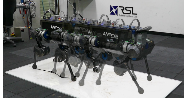
Fig. 1. The quadrupedal robot ANYmal tracking an optimized motion plan on a slippery surface. Contact forces are actively modulated to transition between stick and slip phases.
