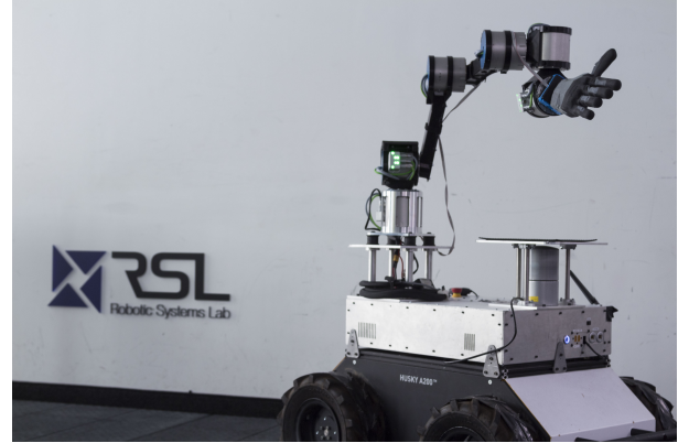
Fig. 1. AnyPulstar, the 6DoF compliant robot used for the experiments and for validating the controller.
