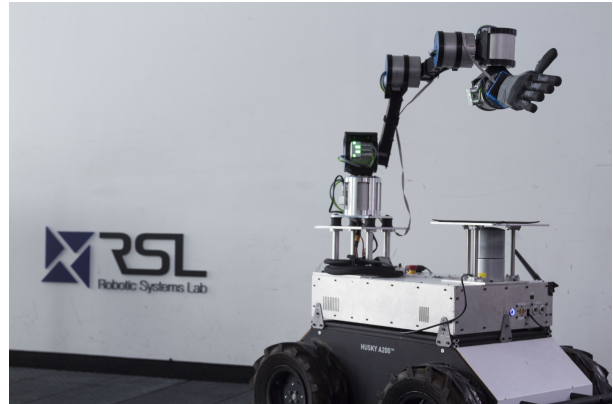
Fig. 1. AnyPulator, the 6DoF compliant robot used for the experiments and for validating the controller.
