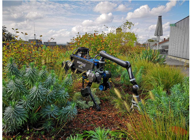
Fig. 1. ALMA, a quadrupedal robot equipped with a six DOF robotic arm. The system is fully torque-controlled, which enables compliant behavior.
