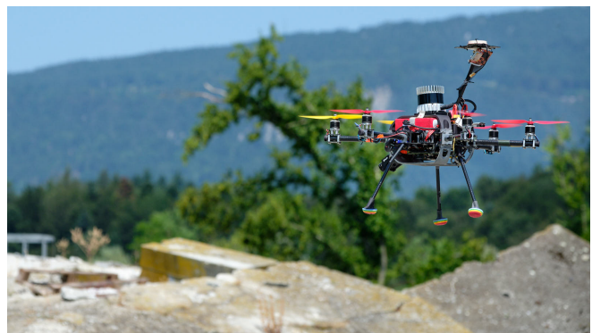
Fig. 5: A hexacopter MAV flying through a search and rescue training area (Sec. VIII-B1). The platform was equipped with a 64 beam lidar (visible), monocular camera, time-synchronized IMU, and RTK-GNSS (used for trajectory evaluation only).
