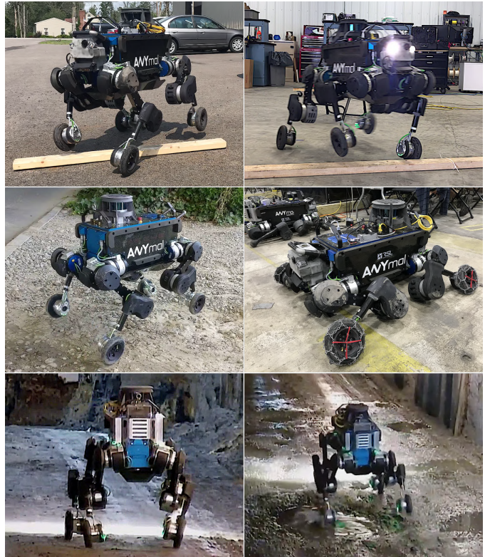
Fig. 1. The fully torque-controlled quadrupedal robot ANYmal [4] equipped with four non-steerable, torque-controlled wheels. The robot is traversing over a wooden plank (top images), on rough terrain (left middle image). In addition, the robot rapidly maps, navigates and searches dynamic underground environments at the DARPA Subterranean Challenge (lower images), and the robot's wheels are equipped with chains to traverse the muddy terrain (right middle image). A video can be found at https://youtu.be/ukY0vyM-yfY .
