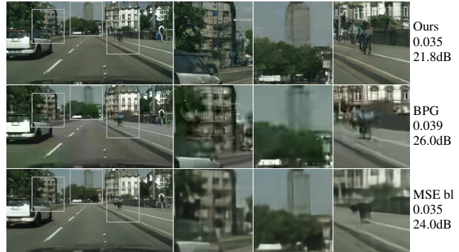
Figure 3. Visual example of images produced by our GC network with C = 4 bottleneck channels along with the corresponding results for BPG, and a baseline model with the same architecture ( C = 4 ) but trained for MSE only (MSE bl.), on Cityscapes . We show bitrate in bpp and PSNR in dB. The reconstruction of our GC network is sharper and has more realistic texture than BPG and MSE bl., even though the latter two have higher PSNR. In particular, the MSE bl. produces blurry reconstructions even though it was trained on the Cityscapes data set, demonstrating that domain-specific training alone is not enough to obtain sharp reconstructions at low bitrates.
