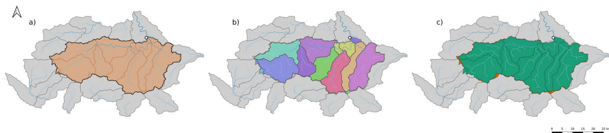
Fig. 4 Visualization of the process of selecting HydroATLAS polygons for deriving catchment attributes for one randomly selected catchment. (a) The orange polygon (bold outline) is the catchment of interest, as represented by a shapefile from one of the CAMELS datasets. Grey polygons (thin outlines) are HydroATLAS (level 12) polygons of the surrounding area. The white dot denotes the catchment outlet (gauge location) and blue lines denote the river network. (b) Shows all HydroATLAS polygons or subsections of HydroATLAS polygons that intersect with the catchment polygon. Note that due to different underlying digital elevation maps, the boundaries of the polygons do not match perfectly. This leads to small intersection artifacts at catchment boundary. To alleviate this problem we excluded small polygons (smaller than 5km 2 ) when deriving the area weighted catchment attributes from HydroATLAS. (c) Shows the excluded (orange) intersecting polygons and the area used for deriving attributes (green).
