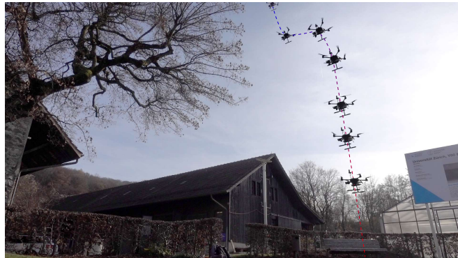
Fig. 1: Safe emergency landing performed during a real-world experiment. Using semantic and depth information, the multi-rotor UAV finds a safe landing area and autonomously descends towards it, while avoiding collisions with the environment.
