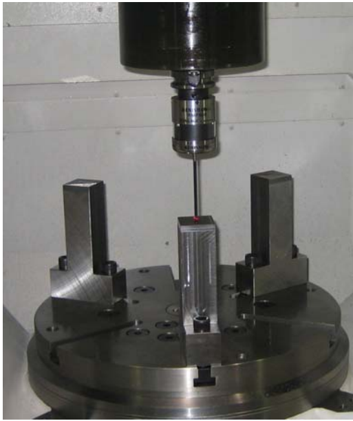
Fig. 13. Setup of three artifacts to calibrate translational and tilt error motions of rotary axes [153].
