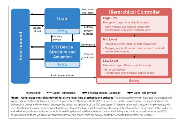
The desired device state is passed to the low-level controller, which computes the error with respect to the current state. It then sends commands to the actuator(s) in an effort to reduce the error. This can be achieved through feedforward or feedback control, and typically accounts for the kinematic and kinetic properties of the device.
