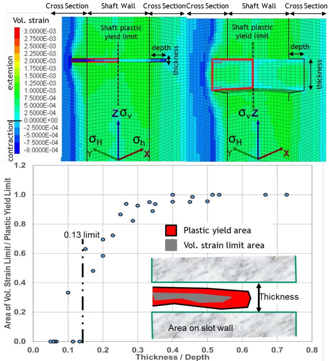
Figure 2. Numerical modelling results from FLAC3D showing relationship between thickness to depth ratio and the area ratio (volumetric extensile strain area to plastic yield area) for slot cut-offs excavated radial from a circular shaft of radius 2.5 m.
