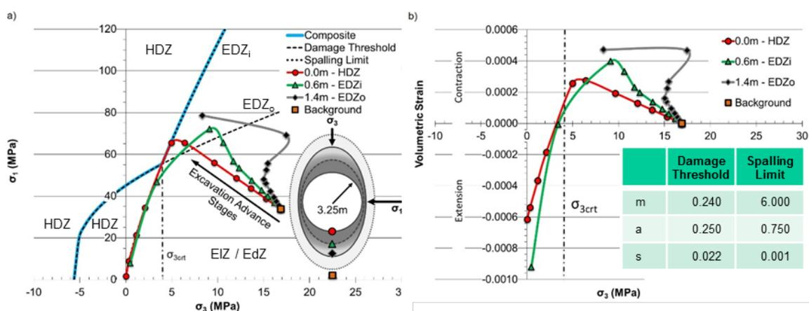
Figure 1ab. Numerical model results from Perras (2014) showing the stress and volumetric strain behaviour of elements within the different excavation damage zones. Inset table of Phase2 input properties to describe the DISL envelops, following method described by Diederichs (2007).
