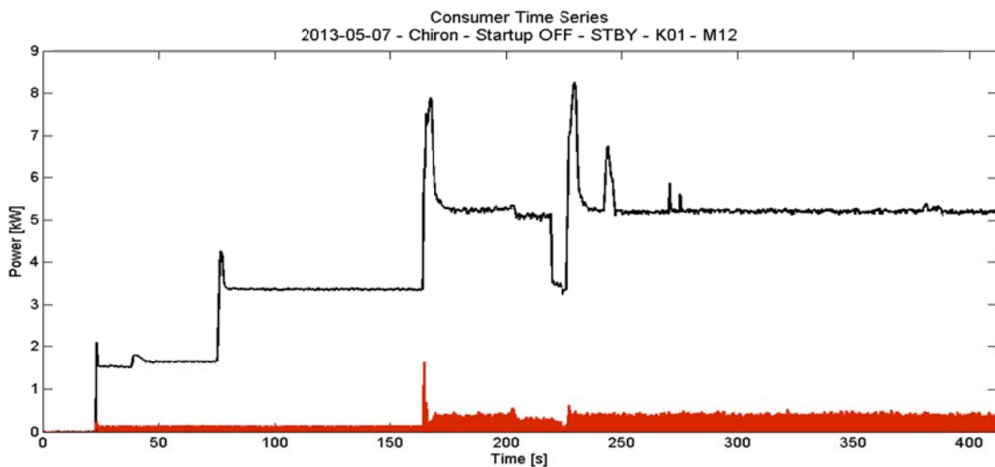
Figure 3.10: Effective power measurement P_{eff,t} on the main supply of the Chiron 12.3W during machine tool startup in combination with the CNC system supply.
