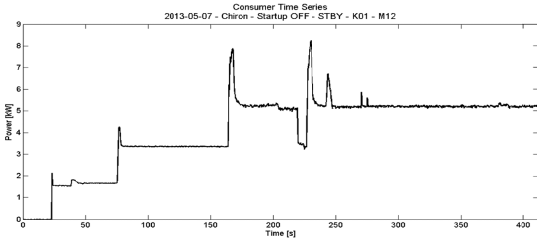
Figure 3.8: Effective power measurement P_{eff,t} on the main supply of the Chiron 12.3W during machine tool startup.
