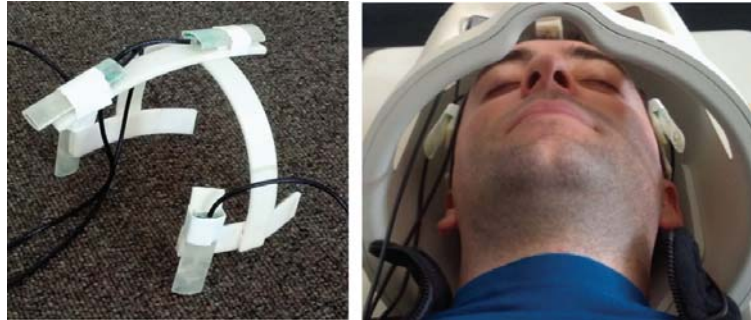
Figure 11: The head setup used for the in vivo experiments. (left) The frame with the four field probes. The probes were attached to the frame with tape, which provided good mechanical stability. (right) The head setup on a volunteer within the head coil used for the in vivo experiments.
