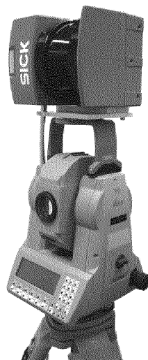
Figure 7.1: Sensor Fusion: Laser scanner mounted on total station.
