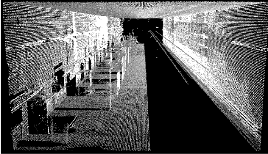
Figure 6.16: Point cloud of test tunnel based on kinematic surveying (inside view).
