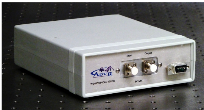
Figure 3.2: 846 nm to 423 nm frequency conversion module. It is a simple fiber-in and fiber-out device for which the temperature of the PPKTP waveguide chip inside needs to be stabilized for achieving the phase matching condition. The SHG temperature coefficient of the module is \approx 0.06 \text{ nm}/^\circ\text{C} .
