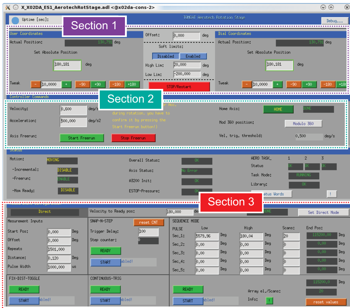
Figure 4.22. Control panel of the Aerotech EPICS driver implementation.
