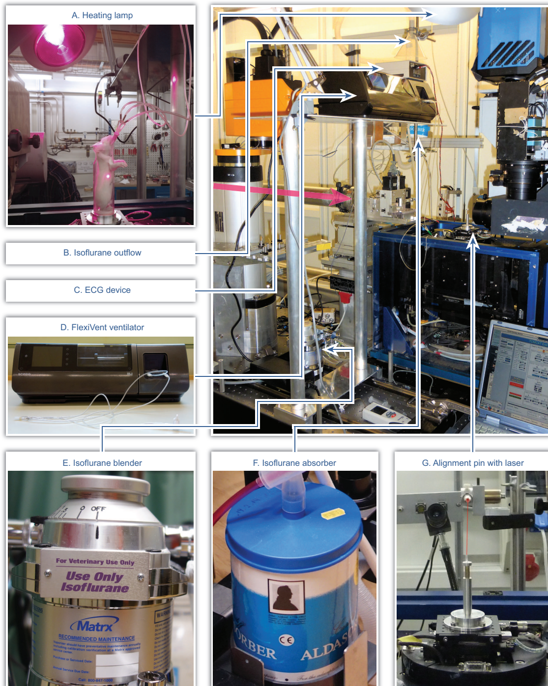
Figure 4.19. In vivo endstation with its main components. The beam direction is indicated from left to right by the pink arrow. Upon the beginning of the imaging experiment, the animal is placed at the position of the alignment pin (visible in A and G). In A, the laser pin light that is used for aligning the region of interest (ROI) is visible, as well.
