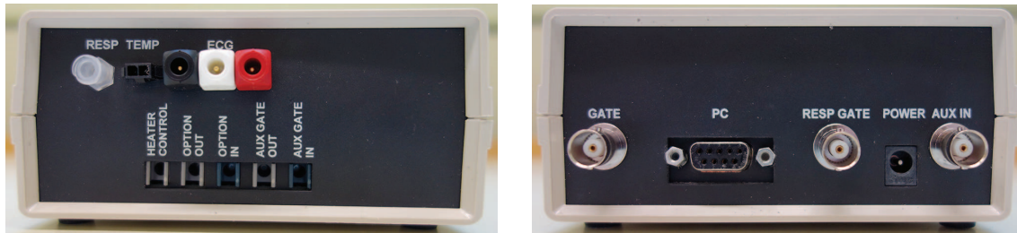
Figure 4.28. Front and rear view of the ECG device with all available connectors. The ECG electrodes, the rectal temperature measurement module as well as the respiration trigger are connected to the front. On the back, the ECG gating signal is available (“Gate”), and the serial connector for the PC controls software is plugged.
