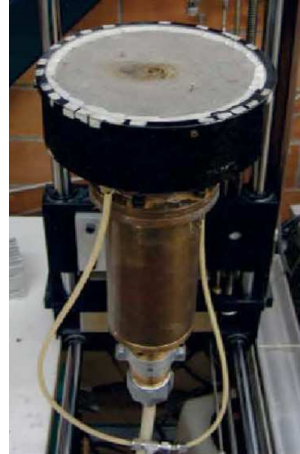
Figure 4.1: The jet burner in (left) a schematic drawing and (right) a side view (showing the porous plate).
