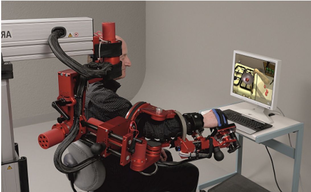
Figure 1.5: ARMin IV shown with a subject performing an activity of daily living training scenario.
