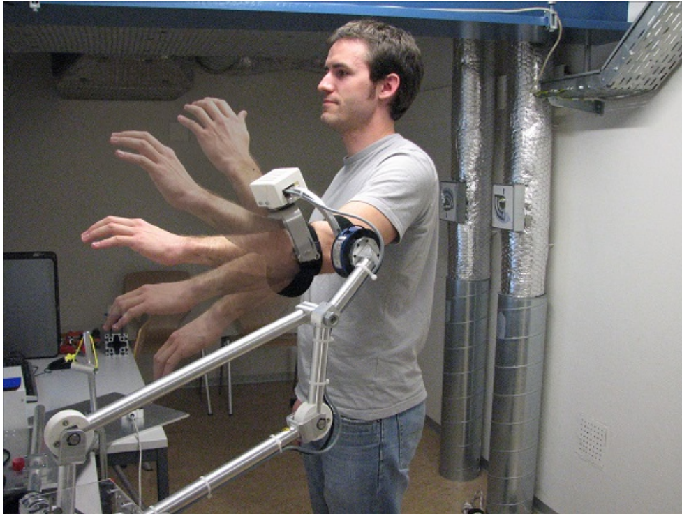
Figure A.1: Visualization of different arm postures that can be reached in a steady robot posture.
