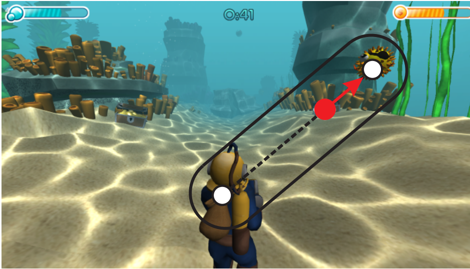
Figure 3.28: Visualizations of the path control strategy for the diver scenario. The diver is walking on sea ground, collecting treasures and air bubbles while shooting pirate fishes and obstacles with his bubble shooter. The AAN path controller supports the hand (target of the bubble shooter) to reach the pirate fishes or the obstacles. Other objects are currently not supported. After shooting a pirate fish or obstacle in the supported mode, the free movement is chosen to let the patient shoot other objects, such as the treasures (e.g., in the left background of the figure) until a new obstacle or pirate fish appears.
