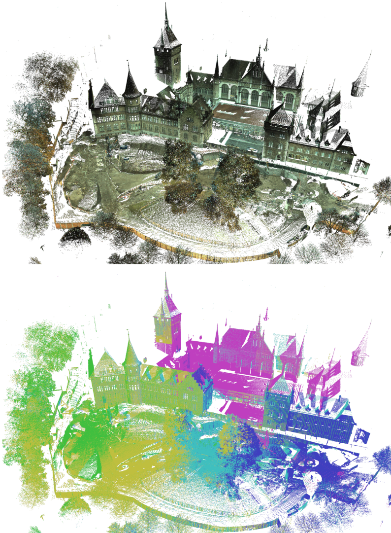
Figure 5.15: Result of our automatic scan registration for CASTLE. The scene was created from 5 viewpoints, color coded in the bottom figure.
