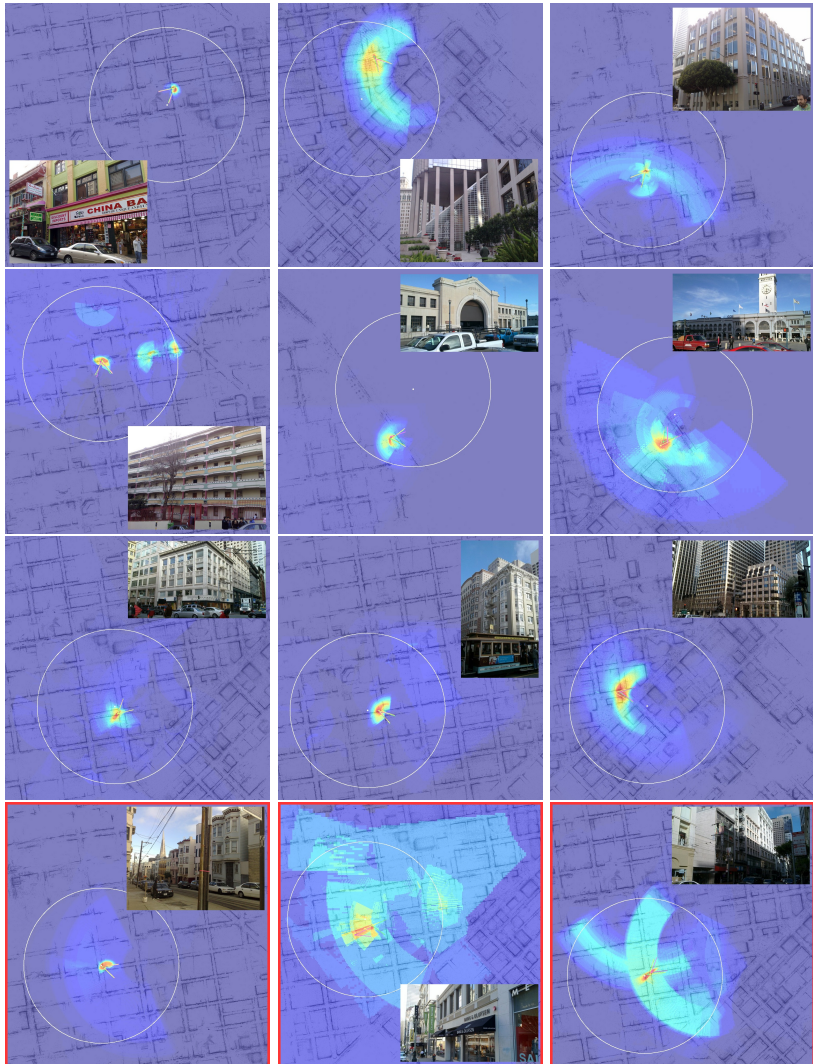
Figure 6.6: Voting heatmaps for different query images of the San Francisco dataset. The first 9 images were localized correctly. Results marked with a red border depict failure cases, where the bottom left denotes a false positive wrt. the ground truth annotation. We believe it is still correctly localized.
