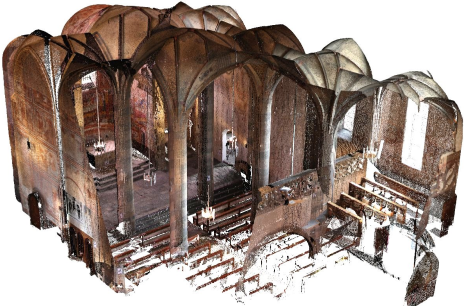
Figure 5.13: Cut through a 3D models obtained by our algorithm from 5 individual scans (CHURCH dataset). We achieve entirely automatic registration of arbitrary geometry from largely different viewpoints by exploiting depth and image data jointly.
