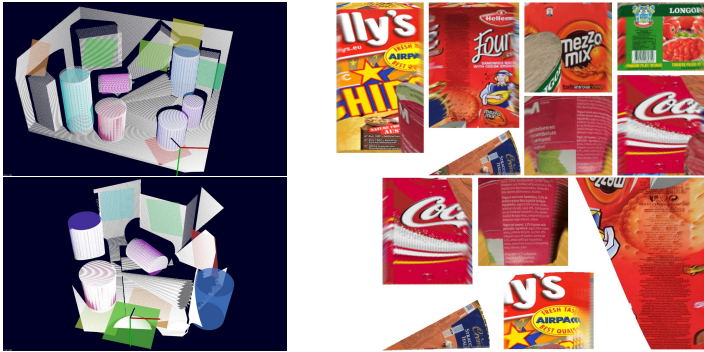
(a) Detected models in the points cloud and their developed surface textures.
