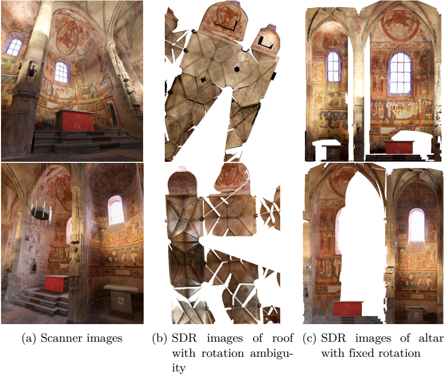
Figure 5.6: (a) Images taken from two different positions, which naturally exhibit a wide baseline. The red altar visualizes correspondence. Feature matching and thus registration from these images fails in most cases. (b-c) Generated salient direction rectified (SDR) renderings along corresponding salient directions. Images of the roof are equivalent up to a 2D euclidean transformation (cf. Claim 2), while images in (c) correspond up to a translation (cf. Claim 3).
