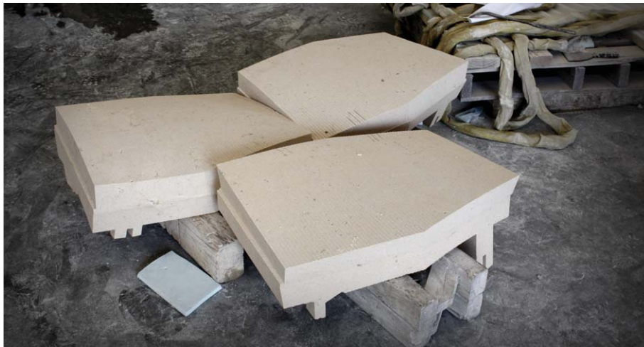
Figure 8.21: Three scaled sample voussoirs of the MLK Jr. Park Vault before undergoing manual surface treatment and assembly.
