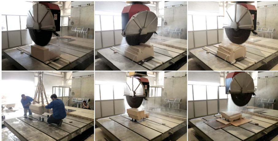
Figure 8.20: From top left to bottom right: sequential stone-cutting process of a scaled sample voussoir of the MLK Jr. Park Vault.
