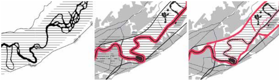
Isère Valley east of Grenoble: river, built areas and floodplain in 1765, 2010, and planned after implementation of the “controlled flood field” (Rossano, from Symbhi, 2009)
