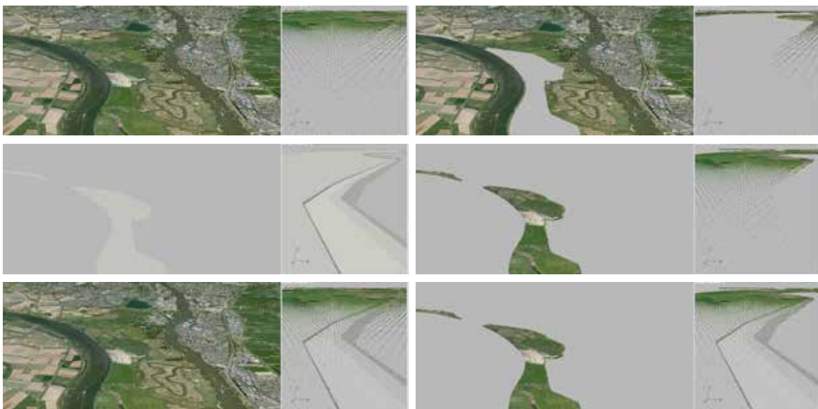
Scenario “extended floodplain”: Modelling and quantifying the volume of displaced ground to restore discharge capacity along the Merwede river (existing levee is displaced and terrain is lowered)
