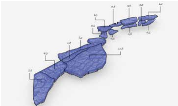
Scenario “fuse polders” in Dordrecht: Evaluation of retention capacity of existing polders (millions m 3 )
