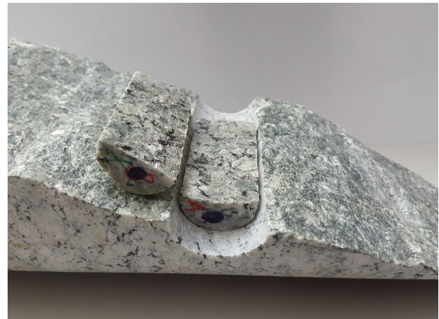
Fig. 1 Example of overcored specimen on top of one fracture surface
