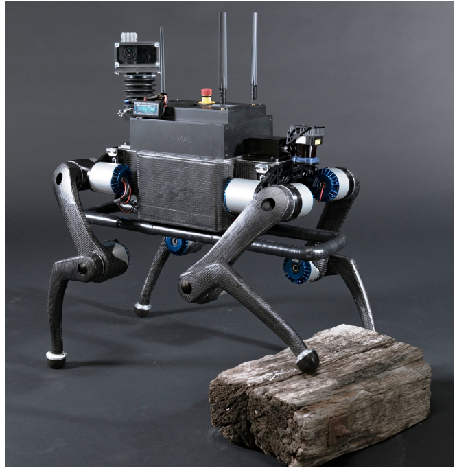
Fig. 1. ANYmal, an autonomous quadrupedal robot for rough terrain operation
