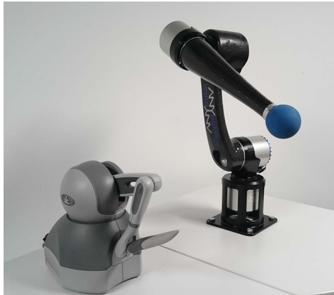
Fig. 1. Geomagic Touch is used for haptic teleoperation of ANYpulator
