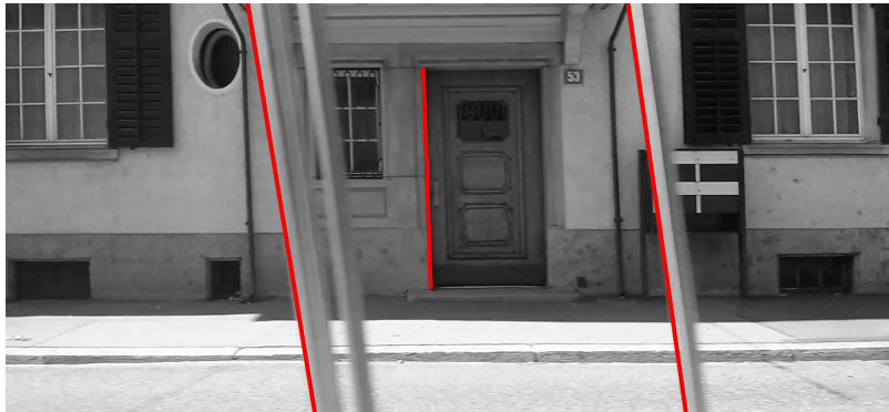
Figure 4.1: Artifacts on an image taken with a rolling shutter camera moving towards the left of the image. The poles and door frame (marked in red), which are supposed to be upright, appear slanted to the left due to the camera motion and the sequential exposure of each scanline from top to bottom of the image. Objects further away from the camera are less affected by the rolling shutter.
