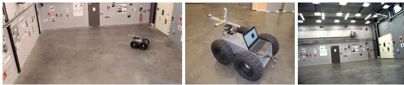
Figure 3.12: Left, Vicon arena used to record the ground-truth dataset. Center, teleoperated Segway mobile robot capturing data. Right, sample image captured by the robot.
