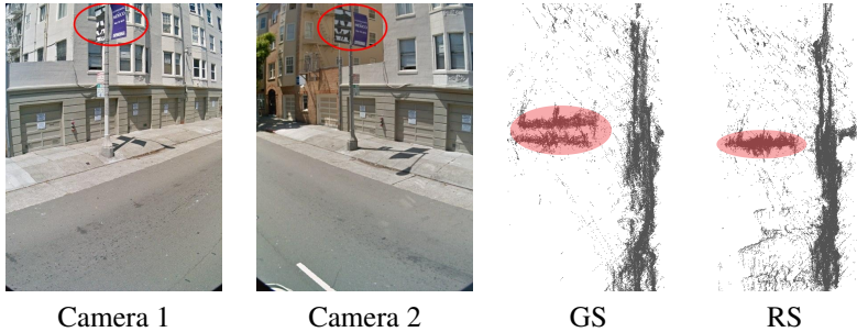
Figure 5.6: Left, sample input image of two cameras mounted on a car. We apply GS and RS stereo on both camera streams independently and fuse the resulting models into a single coordinate frame. Right, bird’s eye view of GS and RS reconstruction. Note how the pole aligns in the RS reconstruction, while in the GS reconstruction it appears as two different poles.
