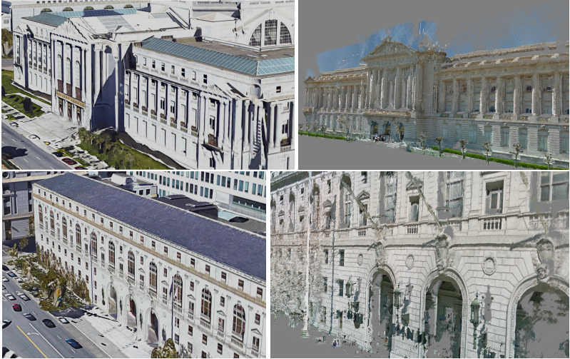
Figure 9.1: Left aerial reconstruction of the San Francisco cityhall (courtesy of google maps). Facades lack geometric details and are approximated as piecewise planar. Right, reconstruction of facade using street level imagery. The model is incomplete (missing roof) but provides detailed geometry.
