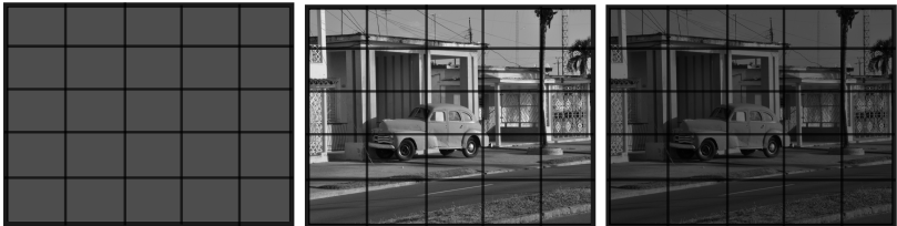
Figure 2.1: Exposure pattern of a global shutter camera. From left to right: First the shutter is closed, then opens up fully to expose all pixels simultaneously. Then the shutter closes again.
