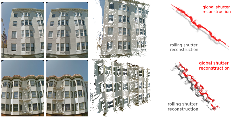
Figure 5.7: Real world reconstruction of the Oak street (top) and Fillmore street (bottom) data sets show systematic differences in bird's eye view (right column).
