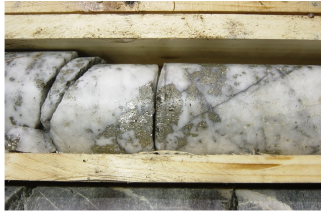
Fig. 5: Drill core of quartz vein with gold and pyrite mineralizations (Dalradian Resources Inc., 2016).
