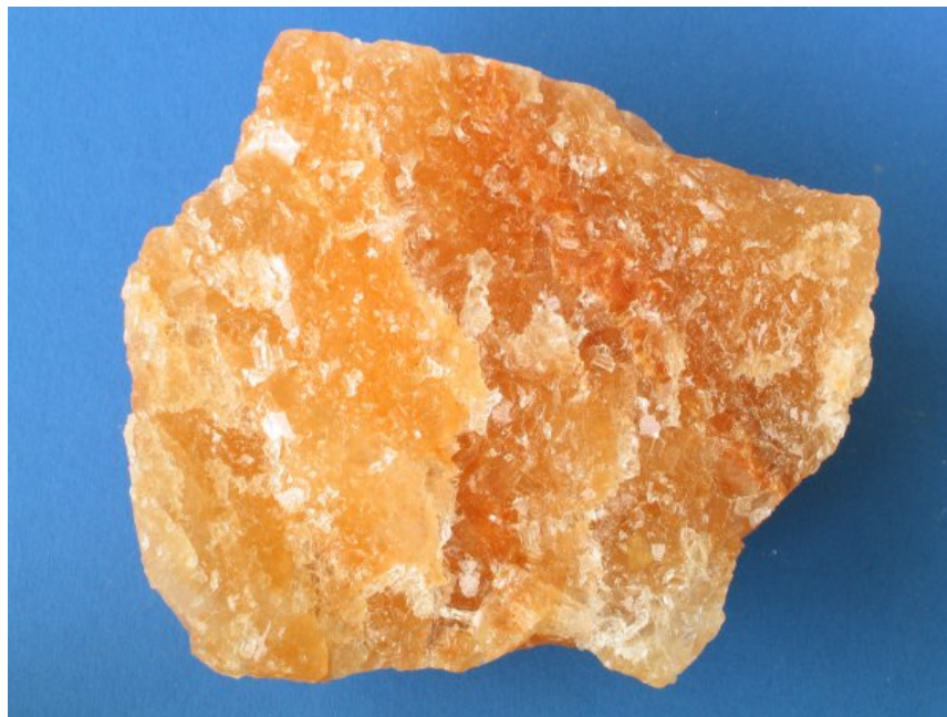
Fig 6: Hand specimen of rock salt, similar to what is mined in Kilroot. Impurities lead to coloring of rock salt. (source: http://www.ifg.uni-kiel.de/Museum/museumsfuehrer/Lagerst/ChemSed.html )
