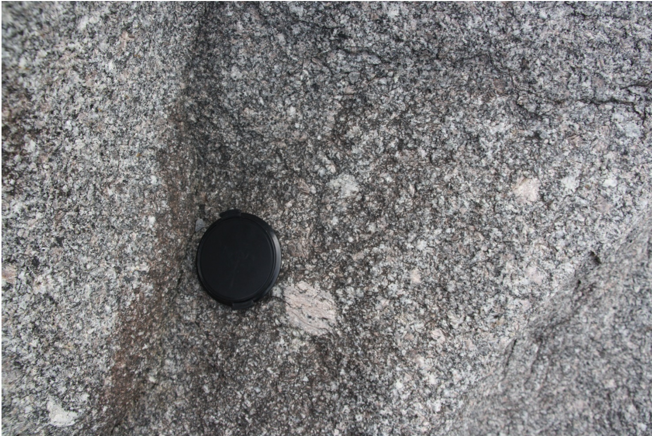
Fig. 2: Primary mineralogy observed: megacrystic K-feldspar, plagioclase, quartz hornblende and lesser amounts of biotite. Secondary mineralogy: molybdenite, epidote, chalcopyrite, fluorite
