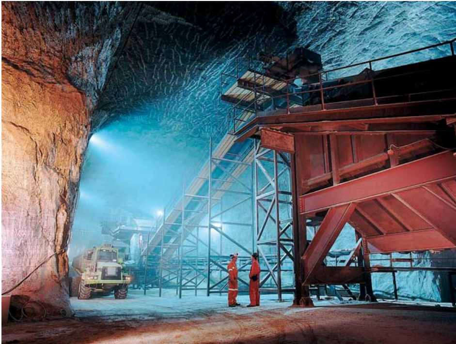
Fig 5: Crushing plant inside the Kilroot mine. The mined rock salt is crushed down to suitable size (about coarse sand), screened, and then transported to the surface with conveyor belts. After treatment with chemicals to prevent baking, it is ready for shipping. Further refining is not necessary, because it is not used as table salt. (sources: see Fig. 4 and http://www.irishsaltmining.com/home.htm )
