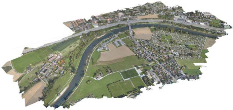
Figure 39 - Processed high resolution digital surface model (DSM) with aerial image texture of an Unmanned Aerial Vehicle (UAV). The data shows a part of the case study area of Schlieren (Canton Zurich, Switzerland) and has an accuracy of 8 centimeters (DSM and aerial image).
