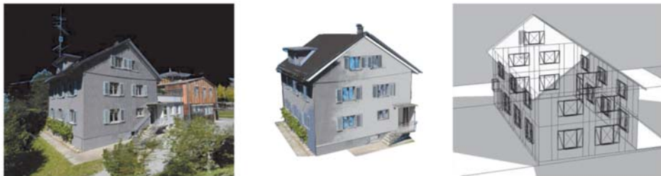
Figure 40 - Colorized point cloud from terrestrial laser scanning (left), static 3D building object model based on point clouds (mid), example of a building type generated in the CityEngine system implementing CGA shape grammar rules (right).
