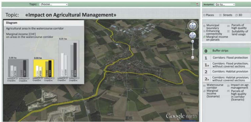
Figure 35 - Information and indicators provided for analyzing effects of watercourse corridor designs on the agricultural production service as monetary benefit for farmers. Spatial visualization of the extent of the corridor according to the flood water protection curve (yellow area) and diagram with correlating quantitative indicators on the total agricultural parcel area located in this corridor as well as the marginal income produced on this area for an ordinary crop sequence and for an extensive management according to the current and potential future agricultural direct payment scheme. (For interpretation of the references to color in this figure legend, the reader is referred to the web version of this article.)
