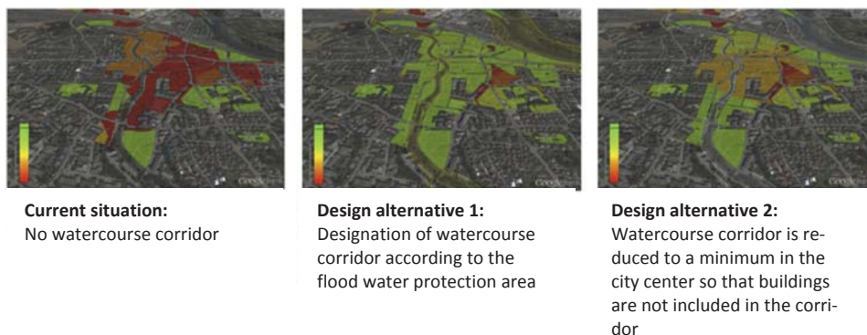
Figure 33 - Indicator maps of the provision of the recreational service of public green spaces for the current situation and alternative watercourse corridor designs: Degree of supply of employees with public open space within a walking distance of 200 m (intense green = 100% \geq 5 m 2 /employee). (For interpretation of the references to color in this figure legend, the reader is referred to the web version of this article.)
