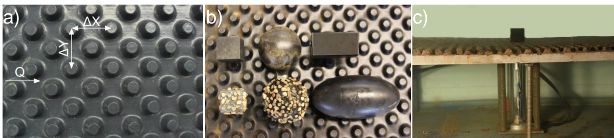
Fig. 1: a) Bed roughness, b) obstacles, and c) installation of the DFS in the flume false bottom.
