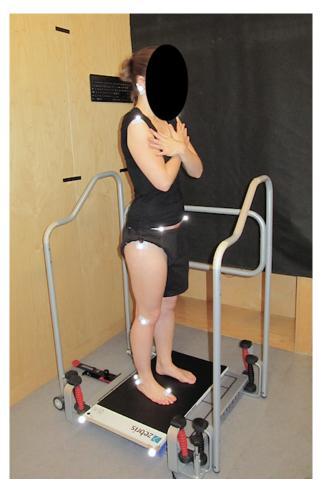
Figure 5.2: Experimental setup: Swaying platform with provocation module and remote triggering from keyboard on wall.
