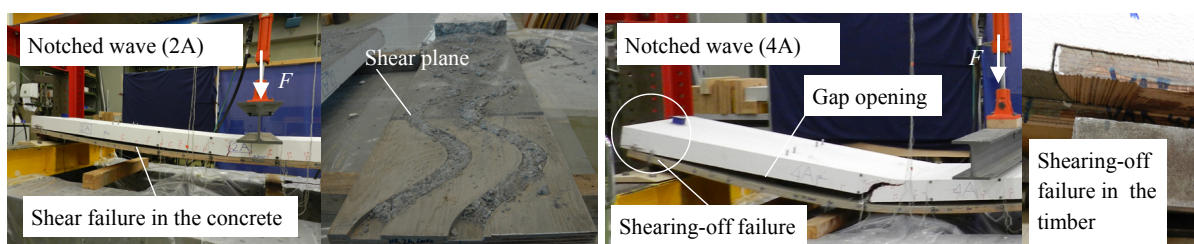
Figure 4.5: Preliminary bending tests: failure modes of the specimens with notched waves
