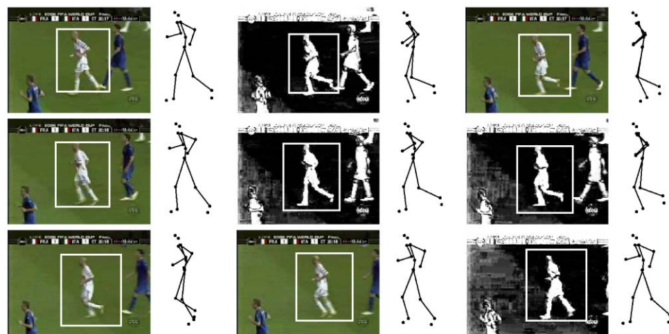
Fig. 5 An extract from a soccer game. The figure shows original and segmented images and with estimated bounding boxes, and estimated 3D poses
