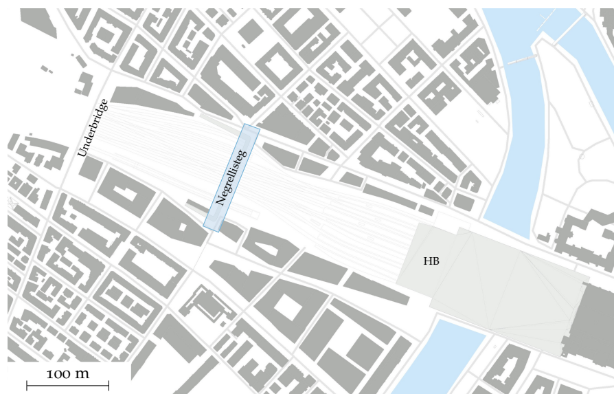
Figure 21: The site of the planned pedestrian and bicycle bridge in the center of Zürich, Switzerland. The blue box indicates the planned bridge called Negrellisteg. The only ways to currently go from one bridge head to the other is by taking the underbridge in the west or going through the main station (HB) in the east.
