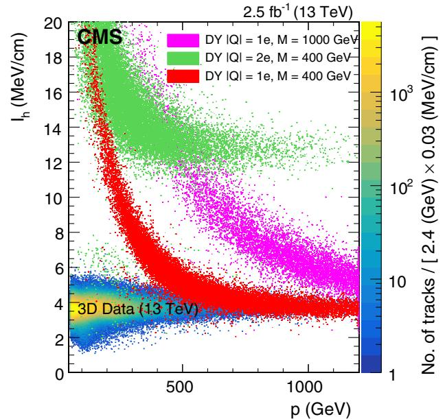
FIG. 1. Distribution of the  $dE/dx$  estimator,  $I_h$  (see Sec. III A), versus particle momentum for tracks in the 13 TeV data, and for simulation of HSCP for singly or multiply charged particles with masses of 400 and 1000 GeV. The vertical scale shows the density of entries for data only.
