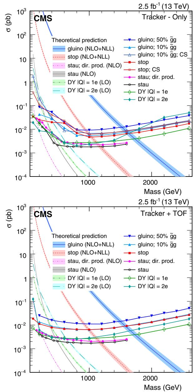
FIG. 4. Results of the HSCP search as the cross section upper limits at 95% CL for various signal models for the *tracker-only* analysis (top) and *tracker+TOF* analysis (bottom) at  $\sqrt{s} = 13$  TeV. In the legend, “CS” stands for charge-suppressed interaction model.
