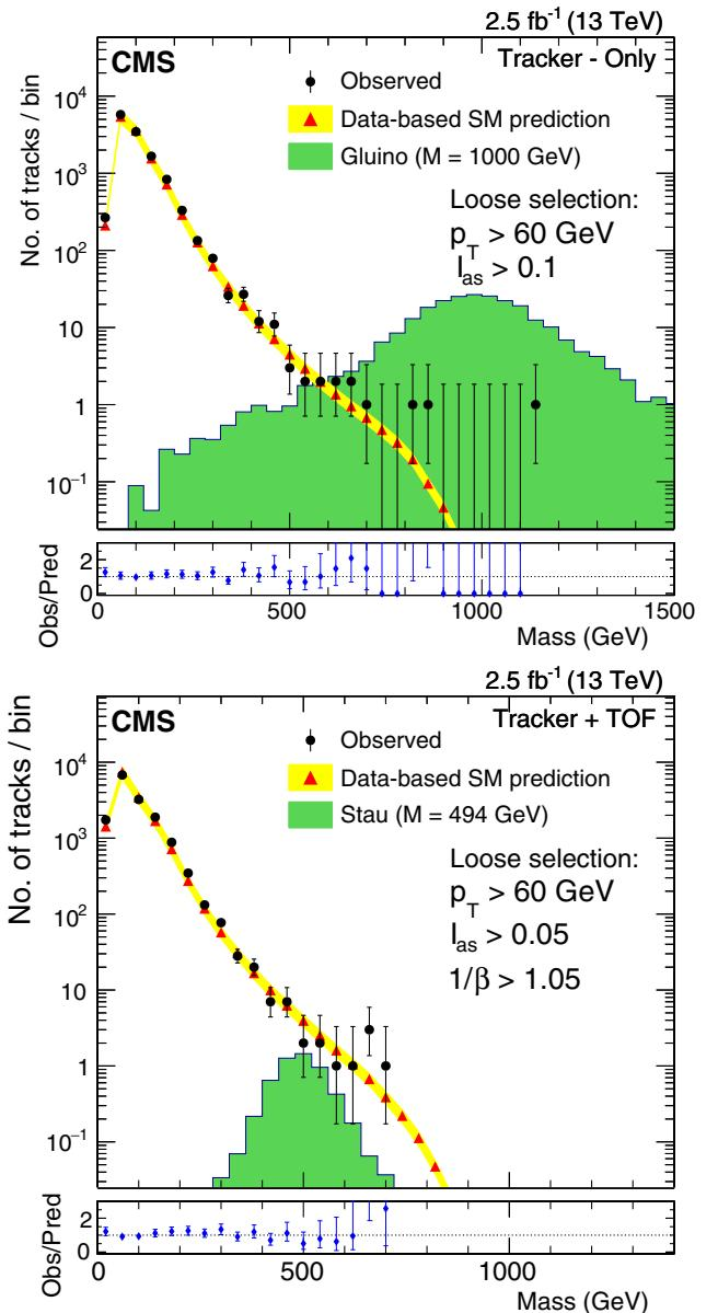
FIG. 2. Observed and predicted mass spectra for loose selection candidates in the *tracker-only* (top) and *tracker+TOF* (bottom) analyses. The expected distributions for representative signals are shown as histograms.
