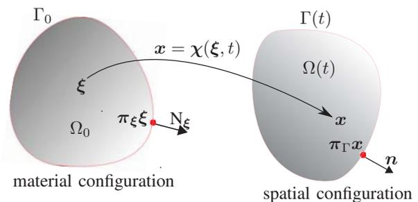
Fig. 1 A sketch for the elastic membrane in material (reference) and spatial (actual) configurations, and forward characteristics in Eulerian elasticity
