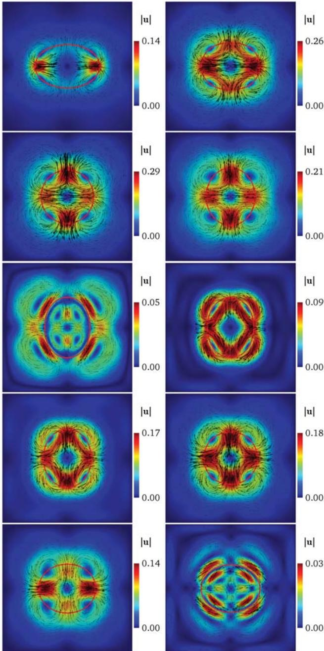
Fig. 2 Snapshots showing the dynamics of the elastic membrane in a viscous flow (shape and velocity profile) at successive times  $t \in \{0.1, 0.48, 0.78, 1, 1.38, 1.6, 1.8, 2.2, 2.5, 2.84\}$ , respectively from top to bottom and from left to right:  $\Gamma$  is plotted with a continuous red line
