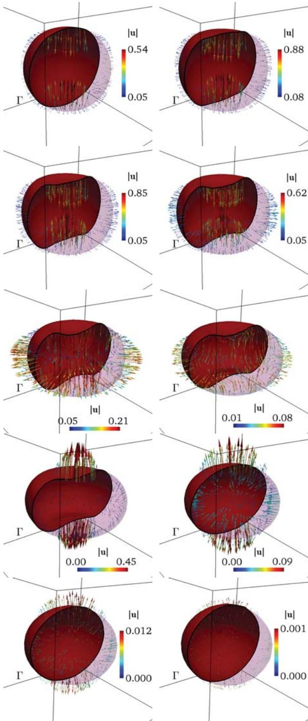
Fig. 6 Snapshots showing the relaxation of an elastic membrane in a viscous flow at successive times  $t \in \{0.06, 0.18, 0.3, 0.4, 0.6, 0.9, 1.32, 1.5, 2, 4.18\}$ , respectively from left to right and from top to bottom: The figures show the velocity field on the membrane  $\Gamma$  (red color)
