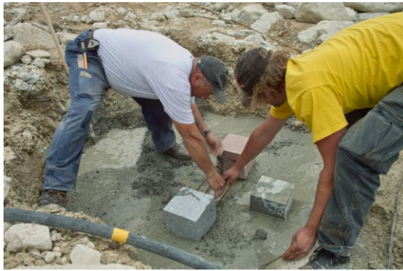
Figure 1. Installation of rock samples at the Illgraben site.
