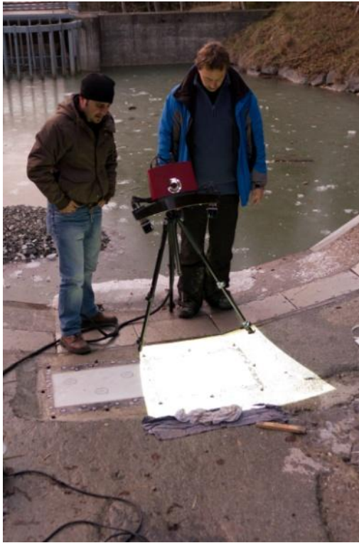
Figure 6. Structured light scanning at the Erlenbach site.
