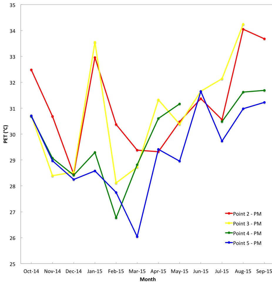
Figure 4.13 – Average PET (°C) values for afternoon hours for all four measurement points.
