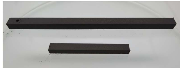
Polycrystalline parts made of powder which was pressed or molded, sintered, and, if necessary, machined
