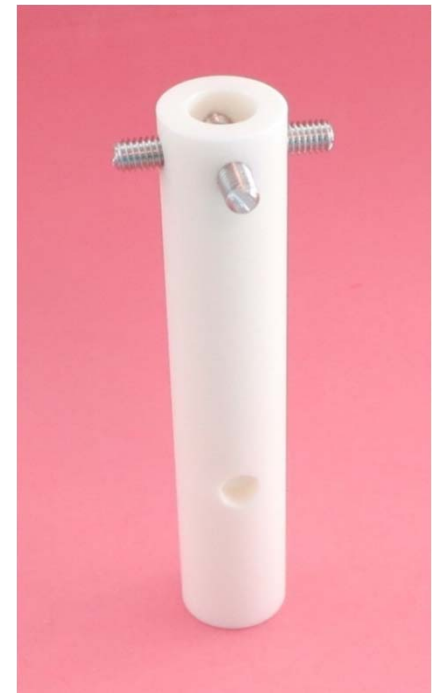
Sample holder with reworked M4 Pt-Rh screws
