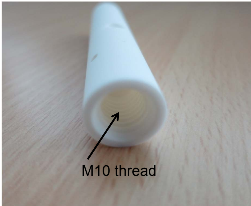
Lower end – can be screwed on the M10 thread of the lower shaft of the mirror furnace
