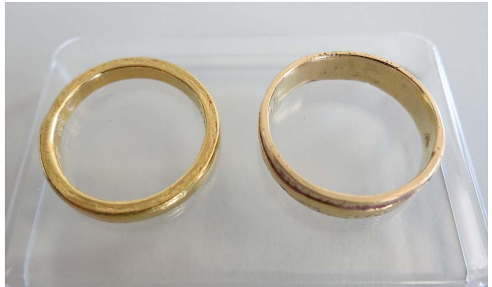
Two rings made of a Rhine gold alloy of the type 750, i.e. they consist of 75 % Rhine gold. The other alloy components are usually silver and / or copper. Diameter about 2 cm. Manufactured in 2013 by goldsmith Karin Demmler in Constance in Germany
