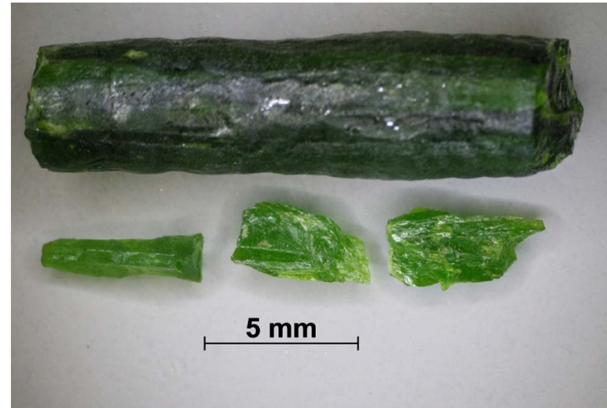
Pr_5Ti_4AlO_{17} = PrTi_{0.8}Al_{0.2}O_{3.40} Pr^{3+} / 4f^2 and Ti^{4+} / 3d^0 structure type n = 5
