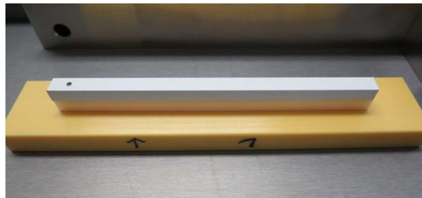
Powder pressed into the form of a 85 mm long rod
