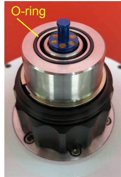
Sample rod and sample inserted into the sample chamber
