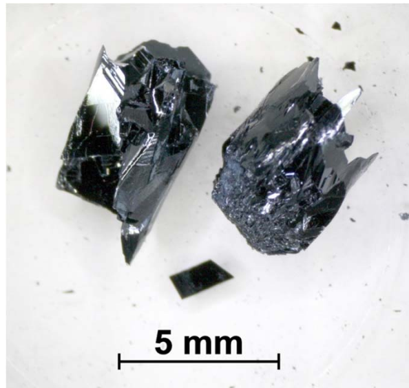
Pieces of as-grown crystalline \text{Sr}_{0.95}\text{NbO}_x . Run / Sample No. 713C
