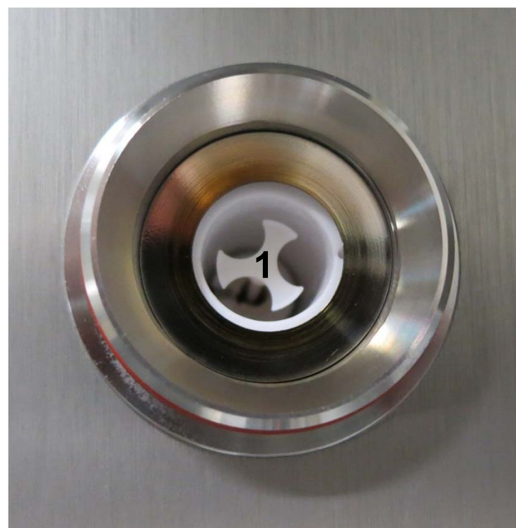
Motor-driven crucible carrier (1) up In this position it can be loaded with a crucible
