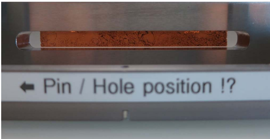
Side view when powder is filled into the pressing die
