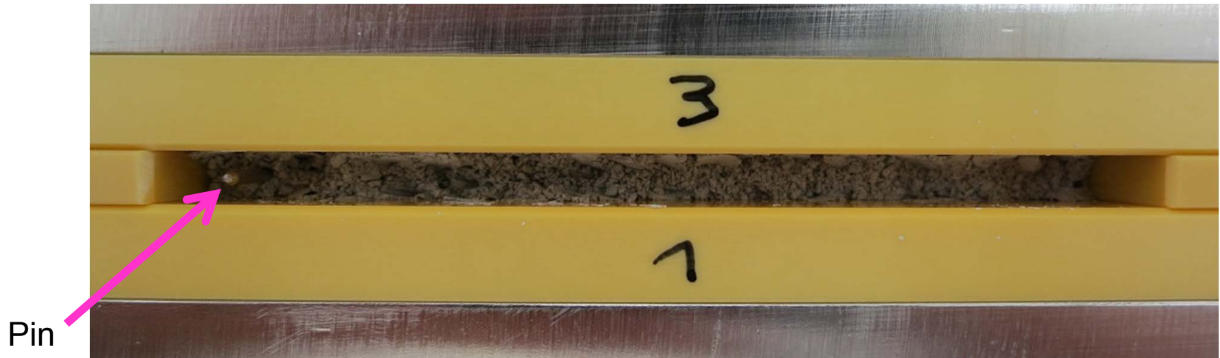
Top view when the lower part of the cavity is filled with powder Chemical composition of the powder in this example: 0,6 \text{ Nb} + 0,2 \text{ Nb}_2\text{O}_5
