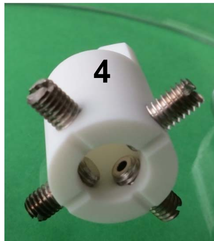
Sample holder made of Macor (4) for the feed rod, equipped with four M4 type platinum-rhodium screws
