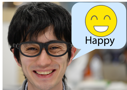
Figure 8. Smart eyewear prototype that is able to recognize emotions by using photo reflective sensors in the frame and machine learning (Masai et al., 2016)
