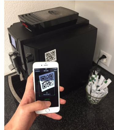
Figure 4. Example of a QR tagged object to invoke a supply reordering service
