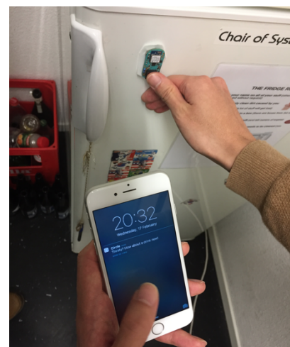
Figure 5. Example of a BLE tagged object with physical button to start the interaction
