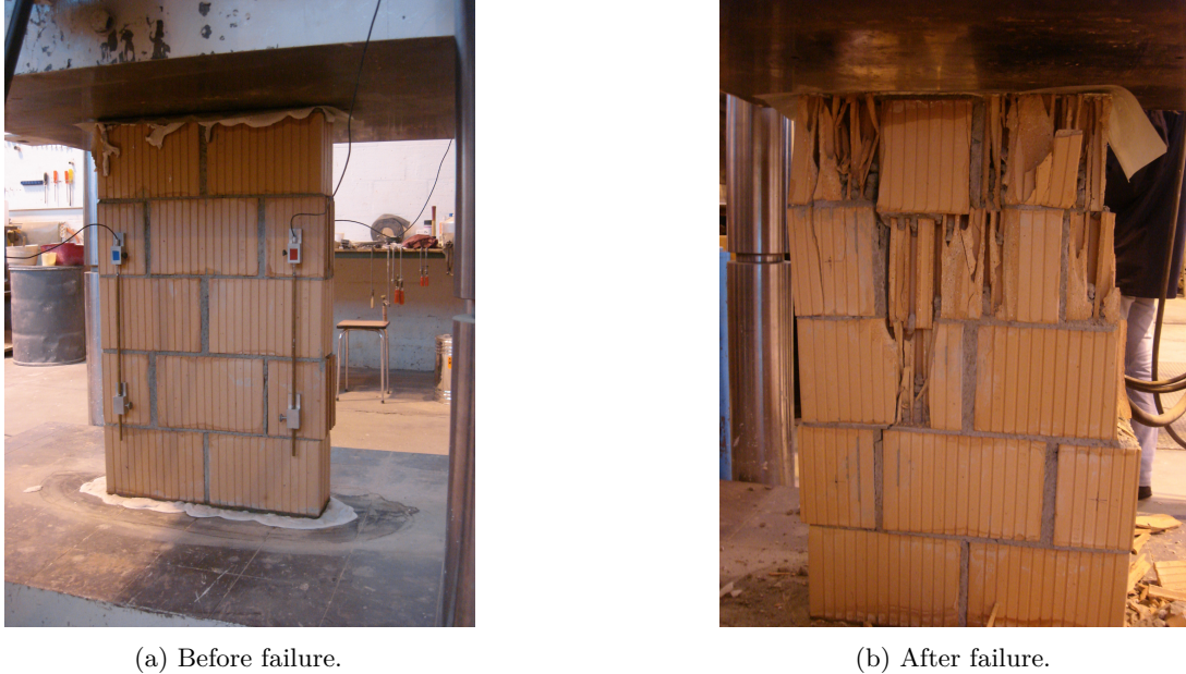
Figure 7.4: Compression test. A specimen is shown before its failure in (a) and thereafter in (b).
