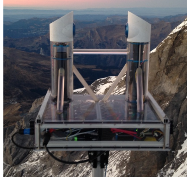
Figure 3. Technical drawing (left) and a picture (right) of the HOLIMO 3G instrument with its main components. The ambient air streams freely between the two towers and the detection volume is the field of view of the instrument between the two towers. The dark blue box indicates the sample volume with the highest resolution ( 6.2\ \mu\text{m} ) and a depth of 75 mm. The dark and light blue boxes indicate the entire sample volume between the towers with a depth of 240 mm. Because the resolution decreases for distances larger 75 mm the minimal resolution in the large sample volume is 20\ \mu\text{m} (Fig. 4).
