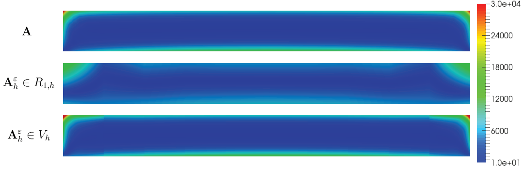
Figure 5.3: Current distribution |\mathbf{j}| = |\omega\sigma\mathbf{A}^{\varepsilon,\delta}| in plate plotted over cross-section y = 0 for \sigma_{\text{plate}} = 5 \cdot 10^7 , \delta_{\text{plate}}/h = 0.063 , k = l = 1
